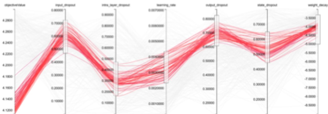
Figure 2: Negative log-likelihoods of hyperparameter combinations in the neighbourhood of the best solution for a 4-layer LSTM with 24M weights on the Penn Treebank dataset.
